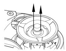
4. Remove the two Drive Pins from the key ways on either side of the Main Shaft.
