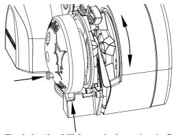
10. Check the 'freefall' feature by loosening the Profish Cap & spinning the Gypsy with your hands. The Gypsy should be able to spin freely.
