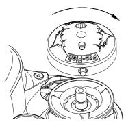
5. Lightly grease the exposed end of the Main Shaft, making sure you **do not** get grease in the threaded hole in the end of the shaft. Place Pro-fish Cap assembly onto the Shaft and screw down by hand.
