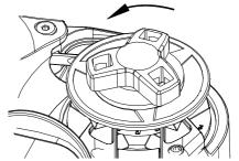
2. Undo the Clutch Nut using 1/2 inch ratchet and or the Pro-Series winch handle & unscrew by hand.
